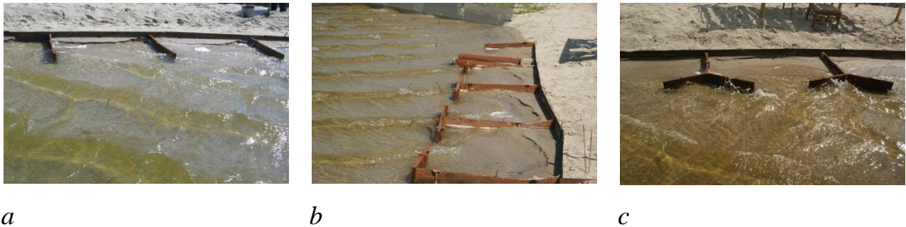
Fig. 1. The models of the coastal protection structures: (a) the groynes; (b) the T-shaped breakwaters and (c) the V-shaped breakwaters with traverses.
