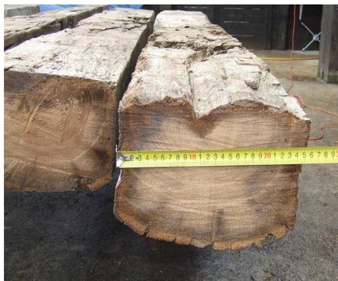
Fig. 1. An example of an oak beam treated with modern tools of a varied structure, covered with a natural patina resulting from contact with weather conditions and the natural aging of the wood. Beam dimensions: length: 2.0 - 4.0 m, cross-section: from 15 x 15 - to 25 x 30 cm. Timber age approx 150-300 years.
