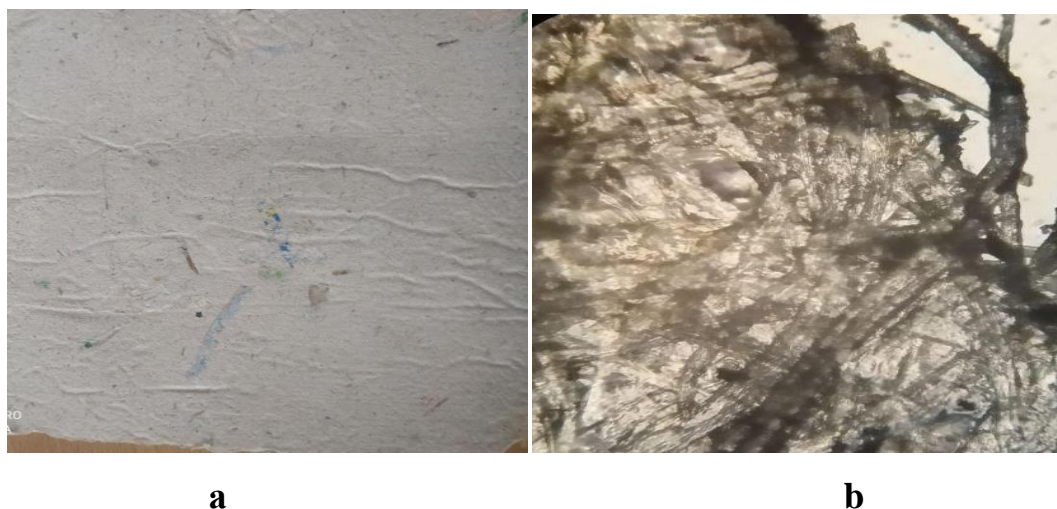
Fig. 3. Photo of the obtained kraft paper (a) and the structure of the fibrous material under the microscope (b)
