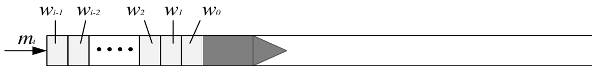
Fig.1. Scheme of formation of the incoming fraction of powder gases at the next step of calculation
