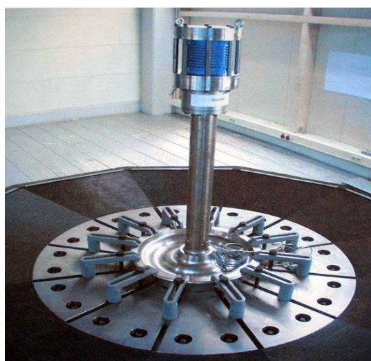
Rice. 2. Stand for dynamic tests on crack resistance of wheels made of R7 steel based on 107 cycles (Deutsche Bahn, Germany)
