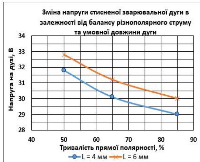
Fig. 2. Change of compressed arc voltage depending on the balance of multipolar current and conditional arc length during plasma welding of aluminum alloy 5154 with a thickness of 7 mm with a frequency of different polar current of 100 Hz.
