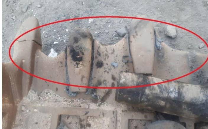
Figure 5. Defect due to abrasion of the cutting edge between the jaw teeth
