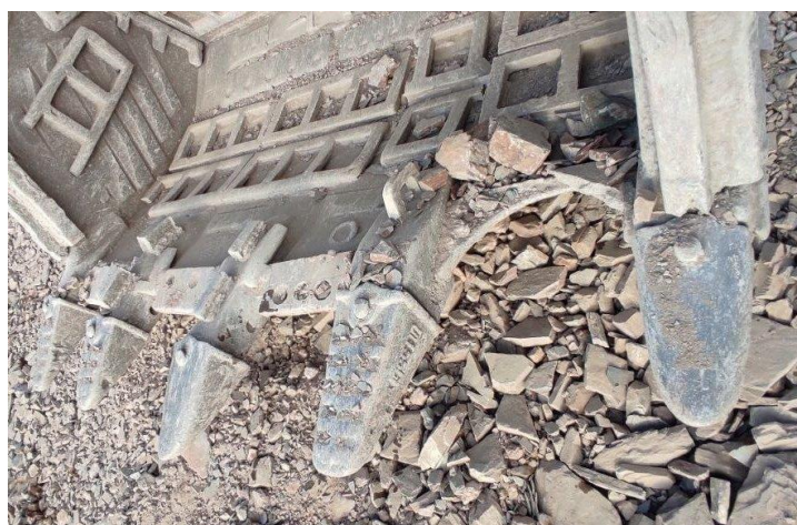
Figure 4: Jaw plate defect in excavator bucket
