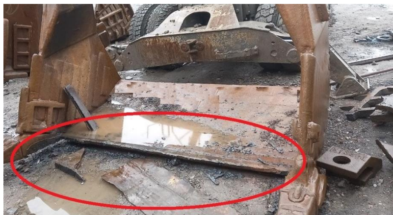
Figure 6. Fracture position of the cutting edge of the bucket's jaw
