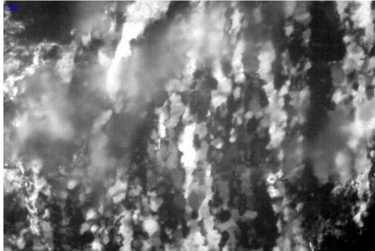
Fig. 4. Quartzite from the Krivoy Rog iron ore basin, metamorphic rock, granular quartz, magnification 100 x
