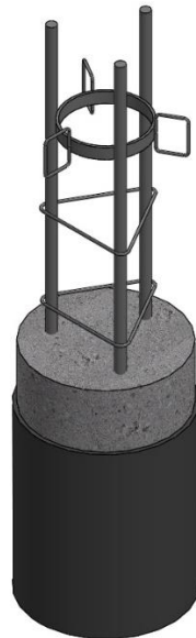
Fig. 3. Reinforcement of pipe concrete pile.
