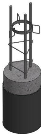
Fig. 3. Reinforcement of pipe concrete pile.
