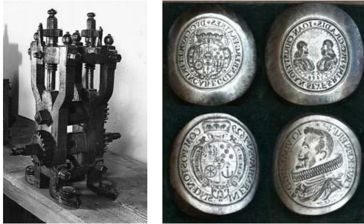
Figure 6. Coining roll with replaceable stamps
