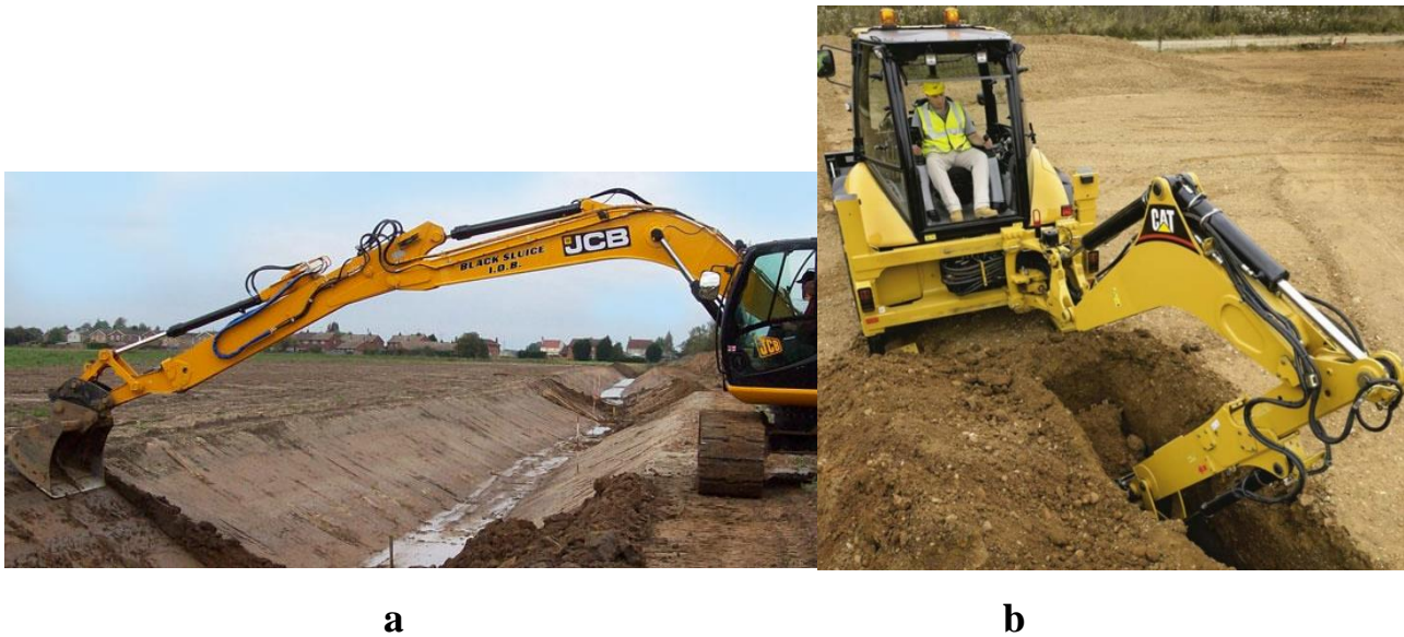
Fig. 7. Excavators with telescopic booms: a) JCB company; b) CAT 444E
