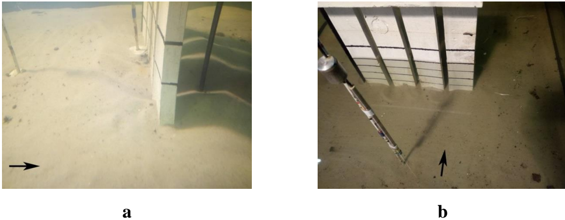
Fig. 3. Erosion and inwash of sandy soil near the slotted breakwater model: side view (a) and view of the sea surface of the breakwater (b)
