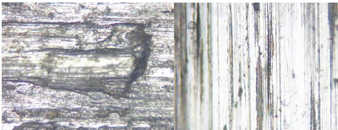
Fig. 2. Condition of the surface of a roller made of steel 25XГ2CPΦ after quenching and high tempering (a) and quenching and low tempering (b) - test for 15 minutes
