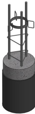
Fig. 3. Reinforcement of pipe concrete pile.
