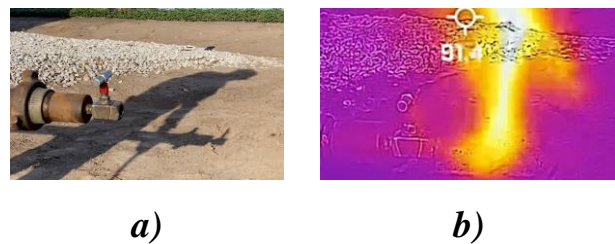
Fig. 4. Foto images B of a transparent flame in normal light (a) and the flame in infrared camera [9].
