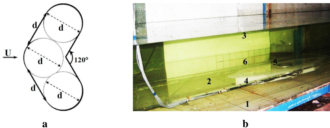
Fig. 1. Scheme of the V-shaped dimple (a) and measuring section of the experimental stand (b).
