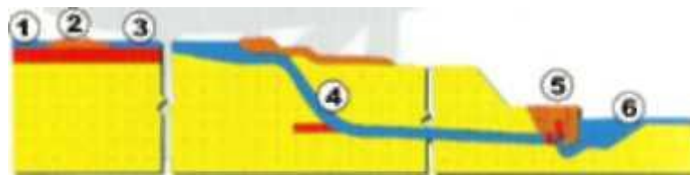
Picture 2. The scheme of TPSPP: 1 – cooling pond; 2 – earthen dam; 3 – upper reservoir; 4 – pressure conduit; 5 – units with hydroelectric generators; 6 - lower reservoir (the Oleksandrivska reservoir)
