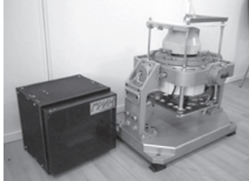
Fig. 3. Gravimetric complex "GREEN-2000/M"
