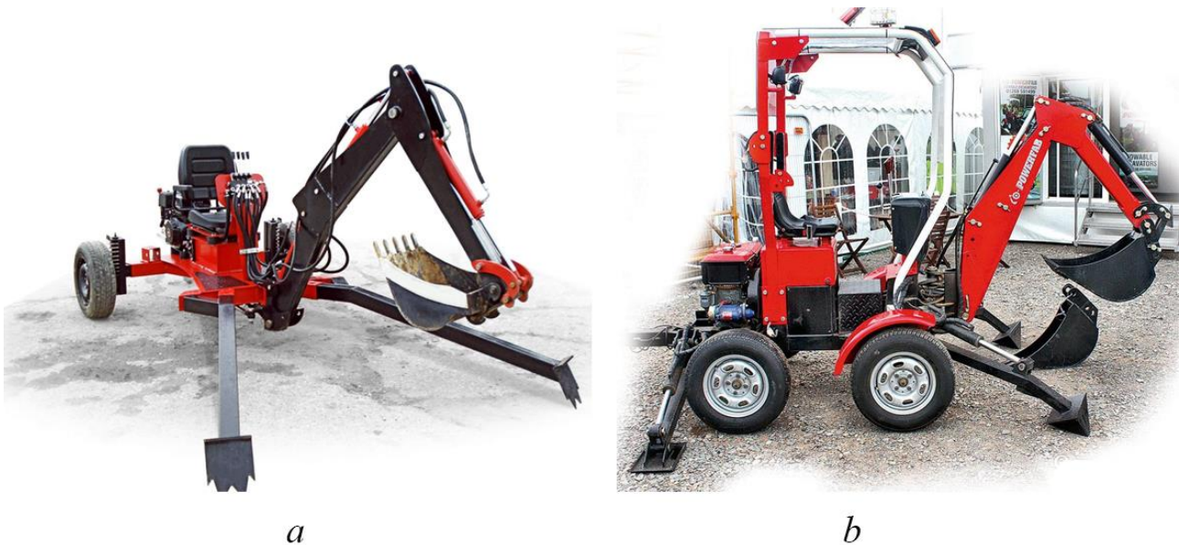
Fig. 1. Examples of trailed excavation equipment in the form of a semi-trailer (a) and an independent two-axle (b)
