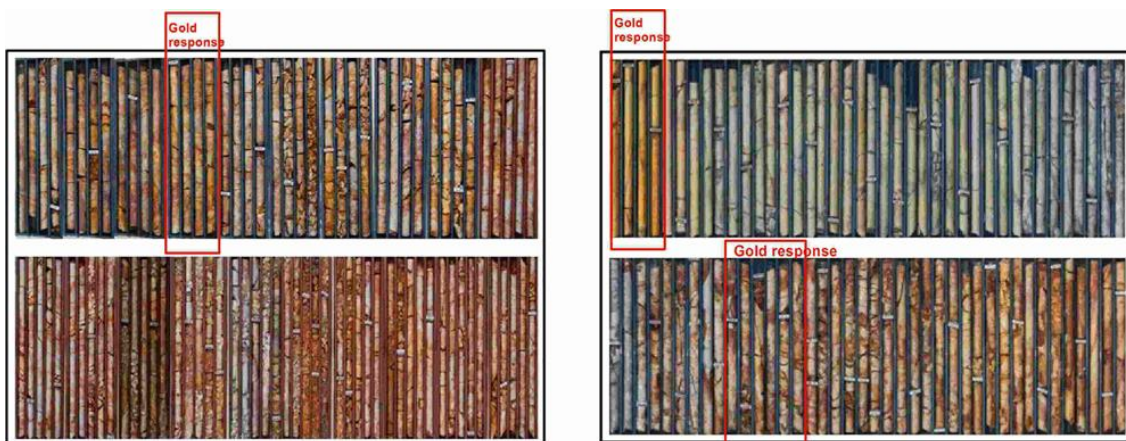
Fig. 1. Core from the wells of the gold deposit [11]. Wells in which the presence of gold is determined by the frequency-resonance method of useful signals detecting are indicated by red rectangles.
