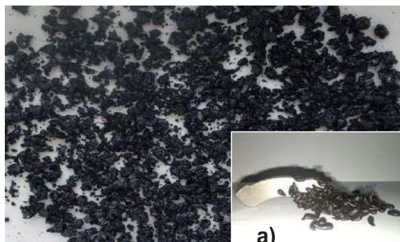
Figure 1. Magnetically controlled biosorbent. a) retention of the sorbent by a permanent magnet.
