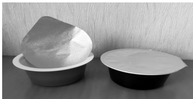
Fig. 2. Polymer container made of multilayer barrier material PET/EVOH/PP with a lid made of aluminum foil with thermoplastic
