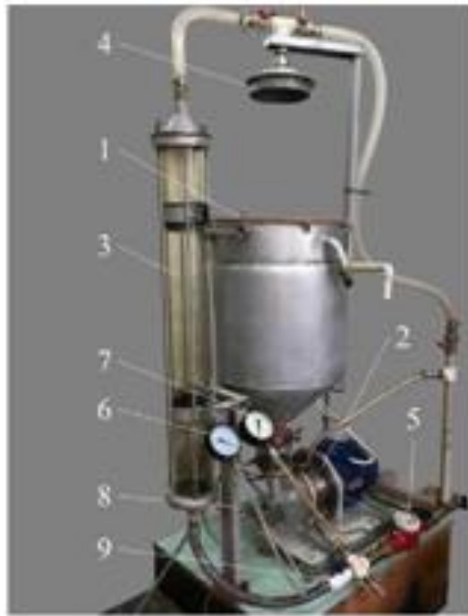
Fig. 1. Rotary-type aeration and oxidation plant (AORT):
