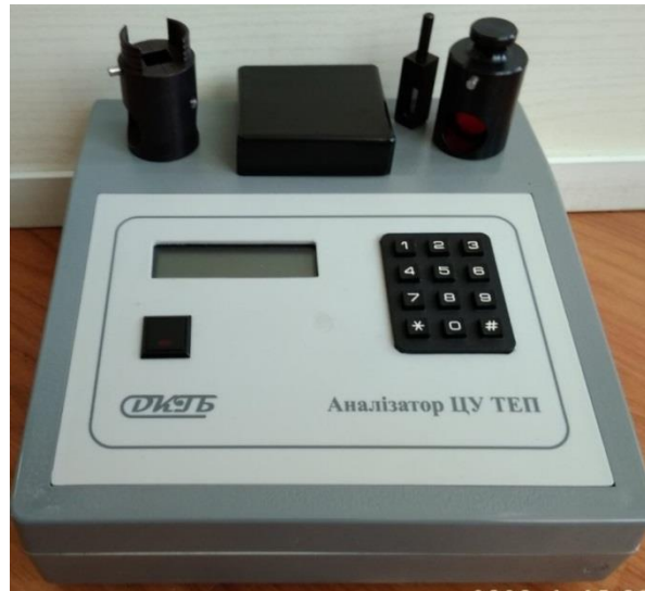
Fig. 1. Automatic TEP-SV-I-6 TEP-SV-I-6 analyzer for operational control of oil product color according to the international Seybolt scale.
