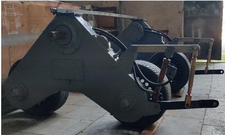
Figure 1. Tandem wheel chassis with suspension mechanisms.
