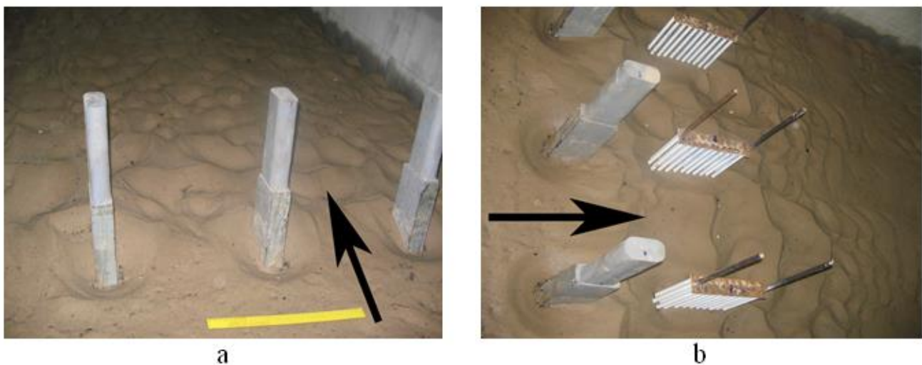
Fig. 1. Bottom topography near a group of prismatic bridge pier models (a) and a group design of two bridge crossing models (b)
