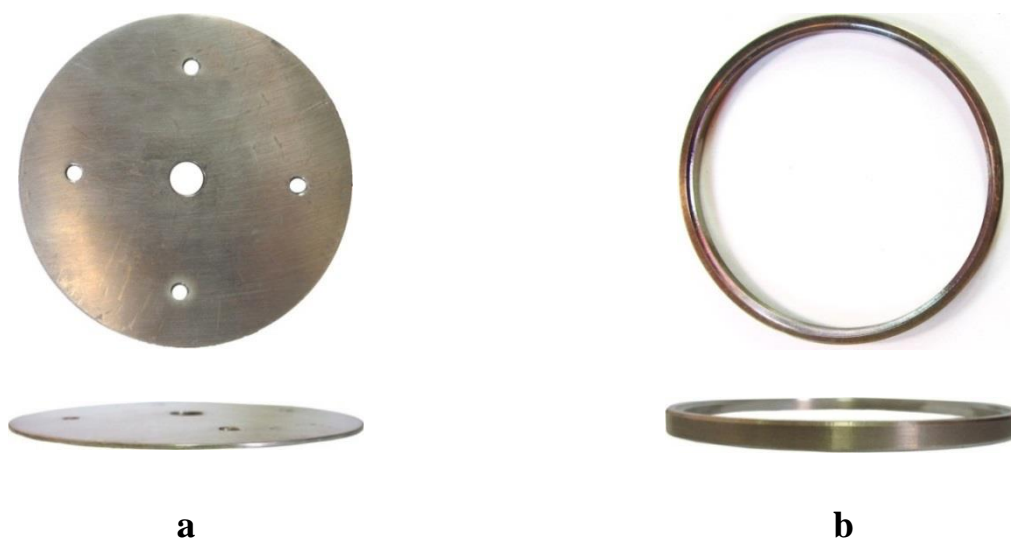
Fig. 1. Components of the deforming element: a – disk, b – ring.
