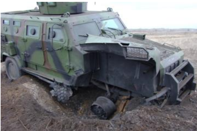
a – explosion beneath the wheel
