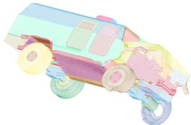
a – explosion beneath the wheel
