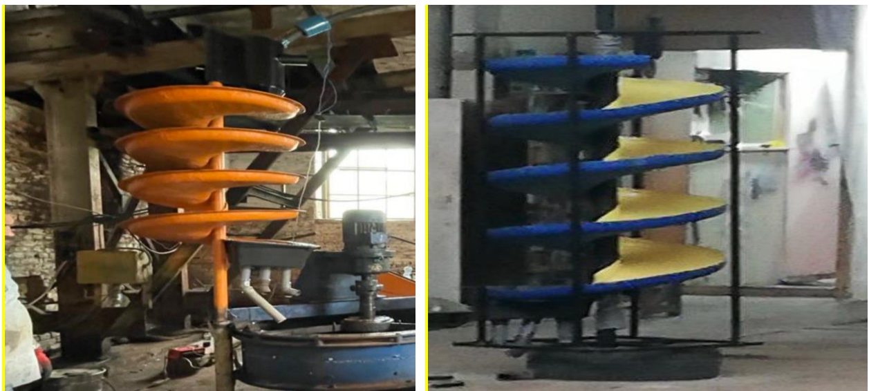
Fig. 1. SVSh-2-1000 spiral separator with different spiral angles
