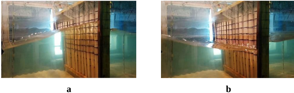
Fig. 2. A 35% permeable wall made of square cylinders with the side facing the wave: crest (a) and trough of the wave (b) in front of the wall
