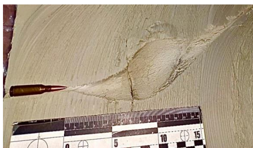
Fig. 4. Damage to the material of the experimental model
