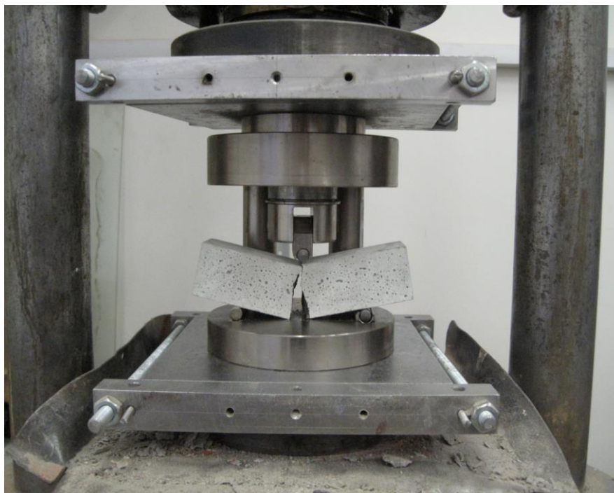
Figure 2. Bending testing of cement samples
