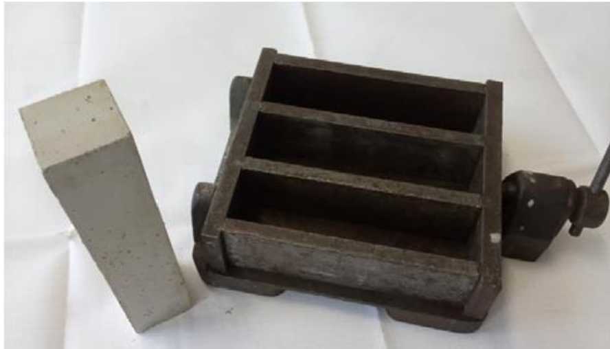
Figure 1. Three-block mold for making beam samples
