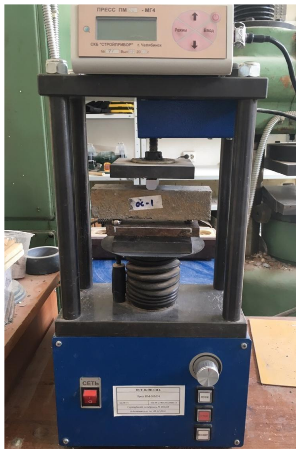
Figure 2. Bending test of beam specimens
